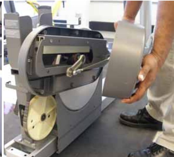
Fig. 4: removing the right outer link cover
