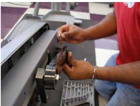
Fig. 7: use the old crank extension mounting bolt
