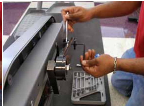
Fig. 8: installing the new control link assembly
