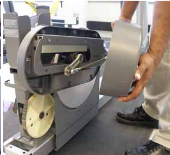
Fig. 4: removing the right outer link cover
