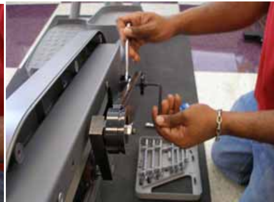
Fig. 8: installing the new control link assembly
