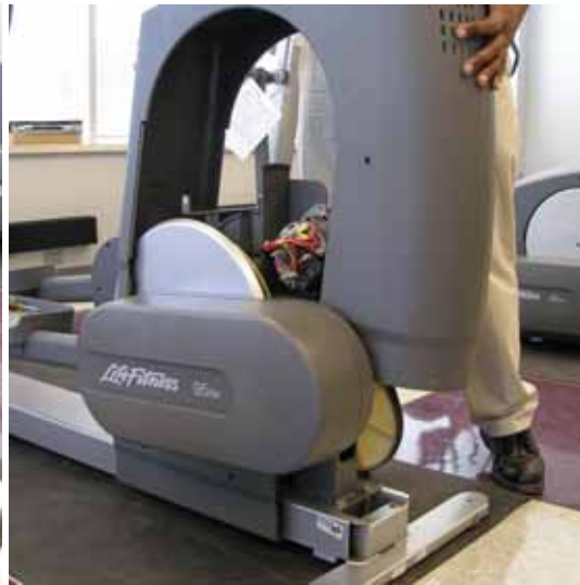
Fig. 2: removing the main shroud
