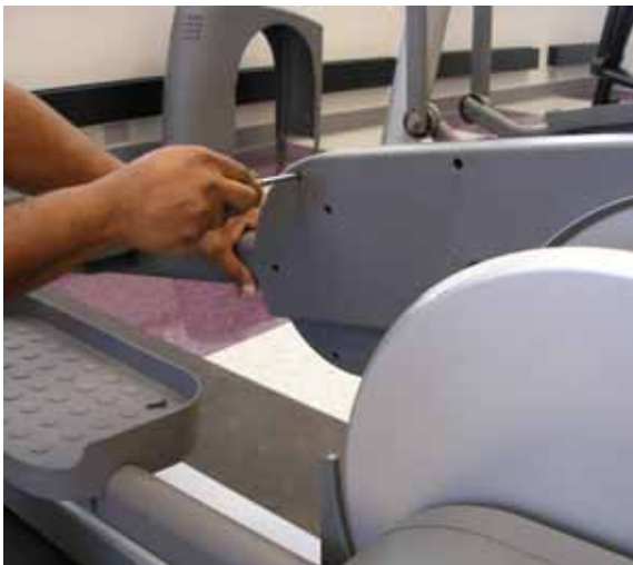
Fig. 3: loosening the right outer link cover screws
